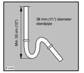
When discharging into a standpipe ensure that the top of the curve in the hose end is no more than 90cm (35.4") and no less than 60cm (23.6") above floor level. The upright standpipe should have a minimum length of 30cm (12") from the bottom of the elbow to the top of the pipe (see diagram).
